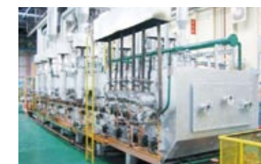
Adoption of mesh belt high-temperature insulation coating for the furnace helped reduce heat loss, leading to a reduction in fuel consumption. As a result, CO 2 emissions decreased by 50 tons per year. (SSF)
