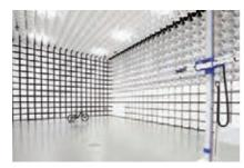
Electromagnetic anechoic chamber
