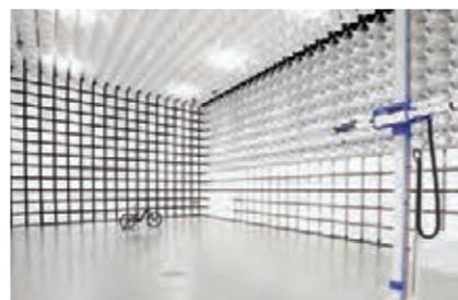
Electromagnetic anechoic chamber
