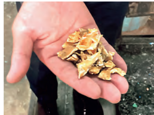
The end-of-life containers are shredded and processed into a secondary raw material for reuse.
